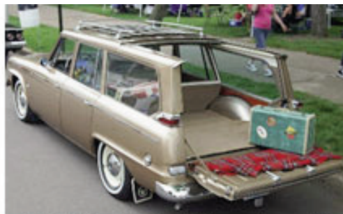
1964 Studebaker Wagonaire with Retractable roof/hinged tailgate
